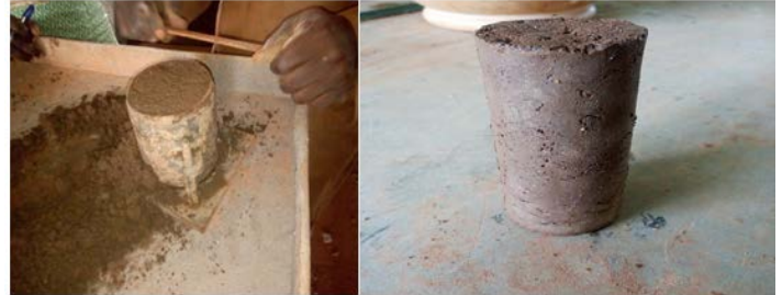
Fig 1: Experimental operation (Compaction and Soil Sample preparation for Triaxial Test)
