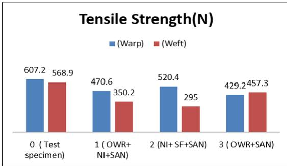
Fig 3: Effect of finishing processes on tensile strength of fabric
