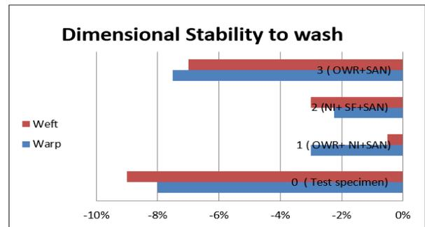
Fig 9: Effect of finishing process on dimensional stability of fabrics.
