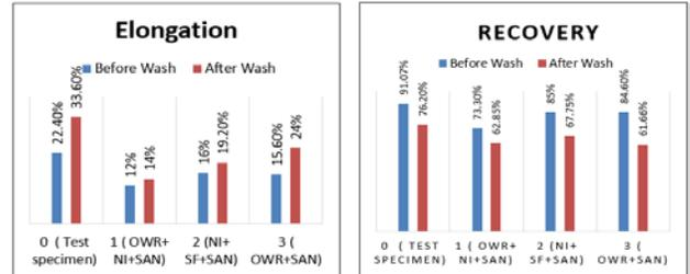
Fig 5: Effect of finishing process on elongation properties
