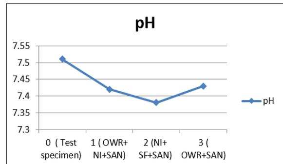
Fig 2: Effect of finishing processes on pH of fabric
