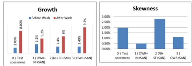
Fig 7: Effect of finishing processes on growth of fabric
