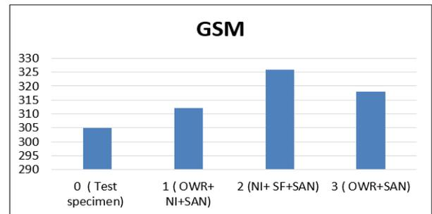
Fig 1: Effect of finishing processes on fabric weight (gm/m<sup>2</sup>)
