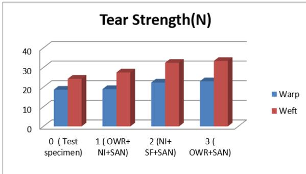
Fig 4: Effect of finishing processes on fabric tear strength
