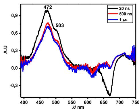
**Figure 3a.** Transient absorption spectra of 2,6-dibromo-1,7-dimethyl-4-hydroxyphenyl-BODIPY in degassed DCM obtained with nanosecond laser after 20 ns, 500 ns, and 1 microsecond after the flash.
