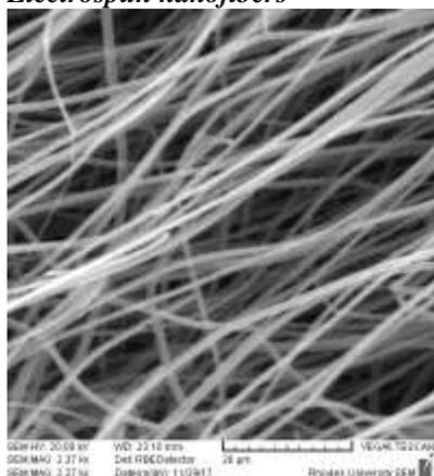
**Figure 4.** SEM micrograph of the functionalized nanofiber mats 25 mg of BODIPY.
