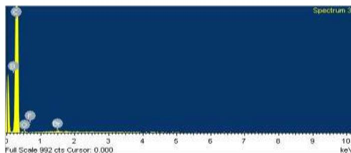
**Figure 5.** EDX spectra of functionalized BODIPY embedded polystyrene nanofibers mats.
