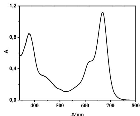
**Figure 2.** Ground state absorption spectra of 2,6-dibromo-1,7-dimethyl-4-hydroxyphenyl-BODIPY in dimethylformamide.
