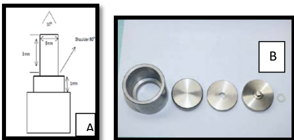
(Figure1) A-master die B- stainless steel mold
