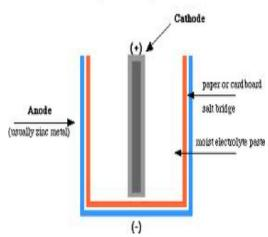
In the most common type of dry cell battery, the cathode is composed of a form of elemental carbon called **graphite**, which serves as a solid support for the reduction half-reaction. In an acidic dry cell, the reduction reaction occurs within the moist paste comprised of ammonium chloride ( $NH_4Cl$ ) and manganese dioxide ( $MnO_2$ ):
