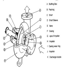
**WORKING:** Like most pumps, a centrifugal pump converts mechanical energy from a motor to energy of a moving fluid. A portion of the energy goes into kinetic energy of the fluid motion, and some into potential energy, represented by fluid pressure (hydraulic head) or by lifting the fluid, against gravity, to a higher altitude.
