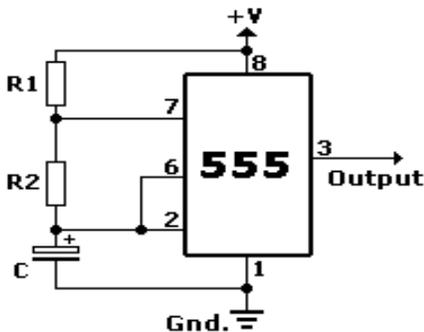
Fig. 6 shows the 555 connected as an astable multivibrator.
