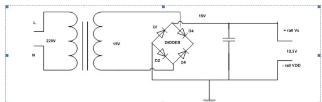
Fig. 8 Power supply Circuit
