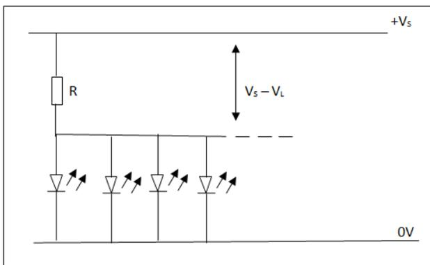
Fig. 9 Light Emitting Diode Unit
