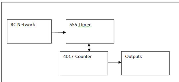
Fig. 2 Block Diagram of the Traffic light controller.
