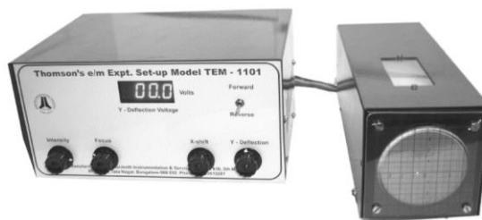
Figure-5: Experimental set-up for determination of e/m
