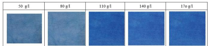
10 g/l of hydrose gives highest depth of shade but this is not used practically as high concentration of hydrose reduces fabric
