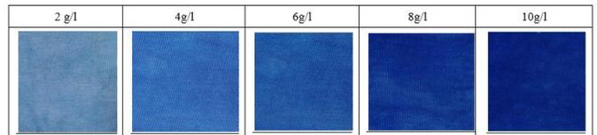
strength [3]. All the performance tests were done on dyed fabric using 140 g/l palm wine and 6g/l hydrose to evaluate dyed fabric quality.
