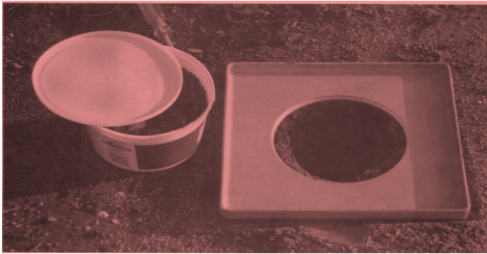
Fig 3.0: Field Density Test on soil (Source: Bardet (1997))
