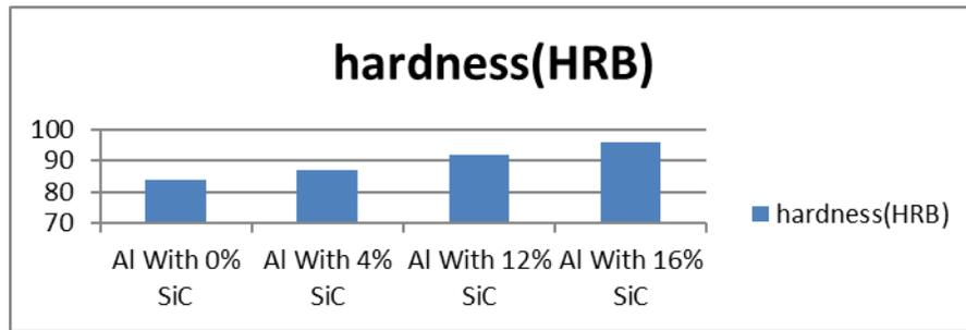
Graph between Wt % of SiC vs Hardness
