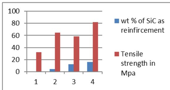
Tensile strength of sic Reinforcement
