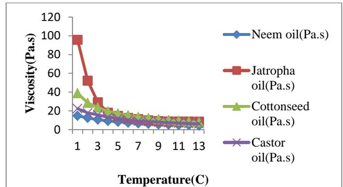
Figure 1: Lubricants viscosity at different temperature ranges from 40°C to 100°C
