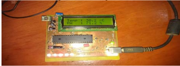
Figure 10: Showing the finished board with all component assembled and tested with temperature reading of 30.2°C and Humidity of 71.2%
