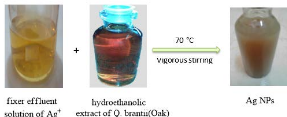
Fig 1. bio-recovery of Ag-NPs from fixer effluent solution of Ag^+ interacted with the prepared peel Oak extract
