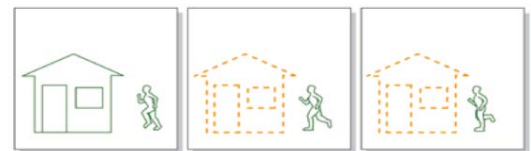
Figure 3.2.4 With difference coding (used in most video compression standards including H.264), only the first image (I-frame) is coded in its entirety. In the two following images (P-frames), references are made to the first picture for the static elements, i.e. the house, and only the moving parts, i.e. the running man, is coded using motion vectors, thus reducing the amount of information that is sent and stored.
