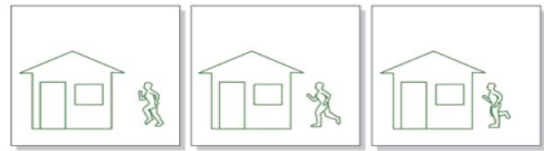
Figure 3.2.3 With Motion JPEG format, the three images in the above sequence are coded and sent as separate unique images (I-frames) with no dependencies on each other.
