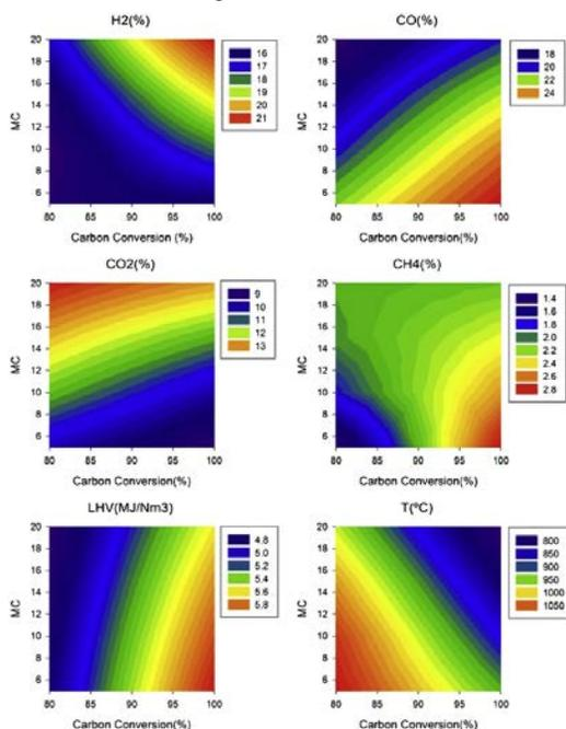
**Fig. 5.** Influence of carbon conversion efficiency on synthesis gas composition and LHV for ER = 0.32.
