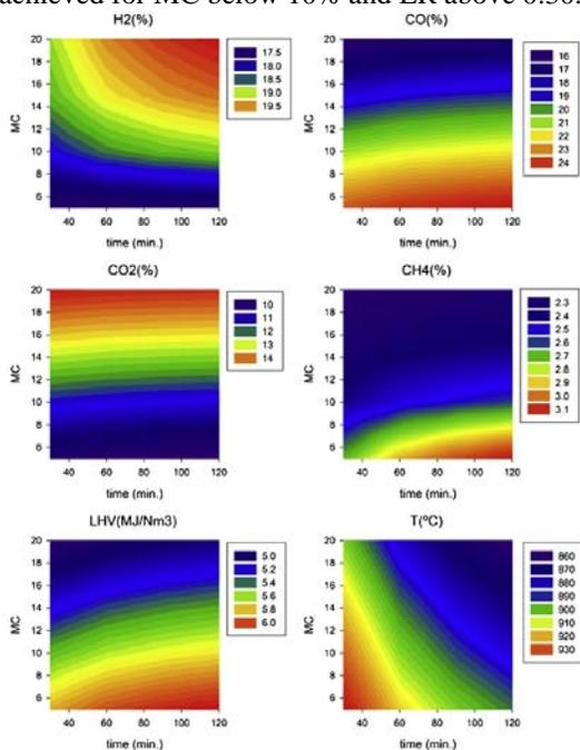
**Fig. 4.** Influence of gasification time on synthesis gas composition and LHV for ER = 0.30.
