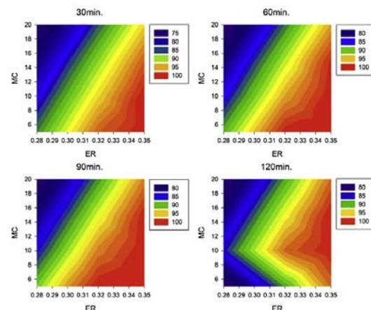
**Fig. 3.** Influence of gasification time on carbon conversion efficiencies.
