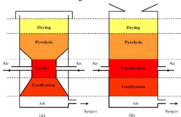
**Fig. 1.** General scheme of downdraft gasifiers: (a) Stratified and (b) Imbert.
