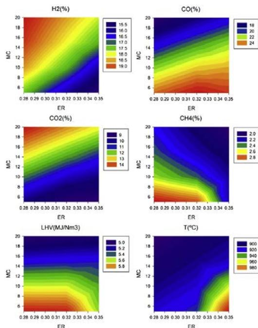
**Fig. 2.** Influence of ER and MC on synthesis gas composition and LHV for 60 min gasification time.
