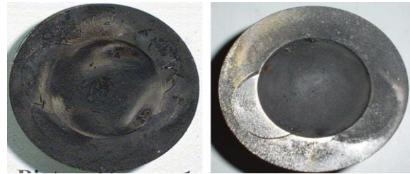
Fig.12 Carbon deposits on piston crown 1) with EGR, 2) without EGR
