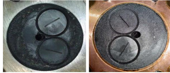
Fig.10 Carbon deposits on cylinder head 1) with EGR, 2) without EGR
