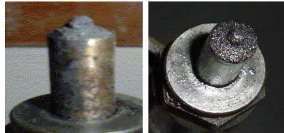
Fig.11 Carbon deposits on injector tip 1) with EGR, 2) without EGR
